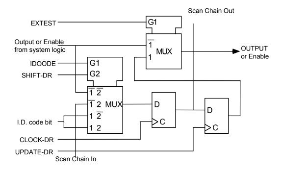
Figure 31 - Bi-directional Cell (IO\_CELL)
