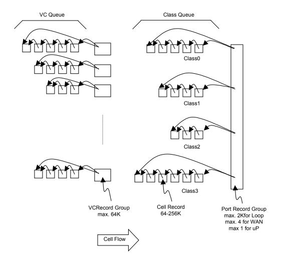
**Note:** The class queue and VC queue as illustrated in the above diagram cannot be directly correlated with the per-Class and per-VC levels as defined in the congestion control.
