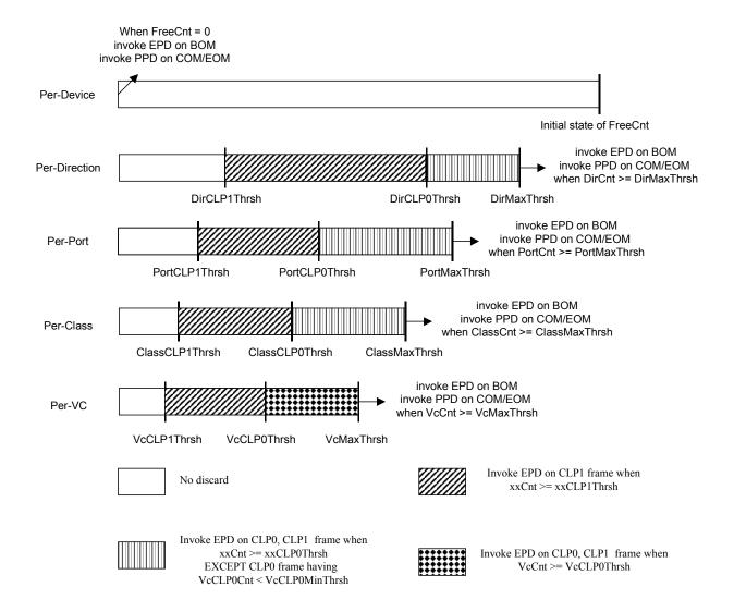
When EPD/PPD discard is selected, the discard mechanism uses the AAL5 EOM PTI field indicator to delineate frame boundaries
