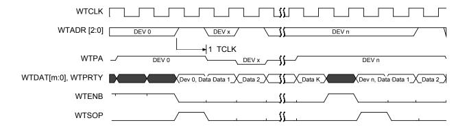
Figure 50 gives an example of the functional timing of the loop transmit interface when configured as a UTOPIA L2 compliant transmit master. It is nearly identical to the WAN UTOPIA L2 transmit master, with the exception of the polling behaviour. Unlike the WAN, the loop interface will assert a NULL address once a
