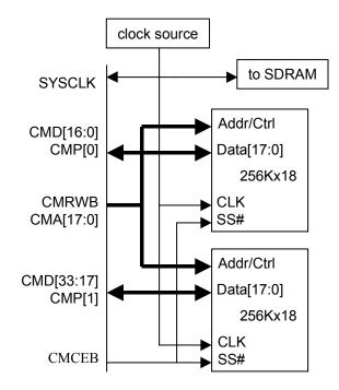
Figure 21 - 2 Bank Configuration for 2MB of ZBT SSRAM
