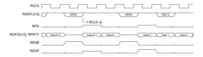
Figure 43 gives an example of the functional timing of the receive interface when configured as a UTOPIA Level 1 compliant receive master. When S/UNI APEX is capable of accepting at least one more cell, and it samples RPA high, a transfer cycle is initiated. If the S/UNI APEX is capable of receiving an additional cell and RPA is sampled high, it will de-assert RENB first before initiating the next transfer.
