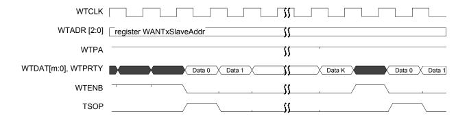
Figure 48 gives an example of the functional timing of the loop transmit interface when configured as a UTOPIA L1 compliant transmit master. It is nearly identical to the WAN UTOPIA L1 transmit master, with the exception that the address on the LTADR bus is indeterminate and should not be used.
