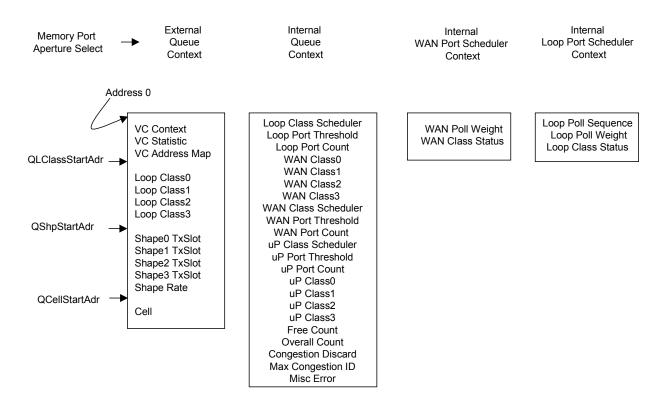
The records for the external context memory are partitioned into four groups: VC, Loop Ports, Shape and Cells. Three registers define the starting physical address of each of the Loop class, Shape and Cell groups, with the VC group always starting at address zero.
