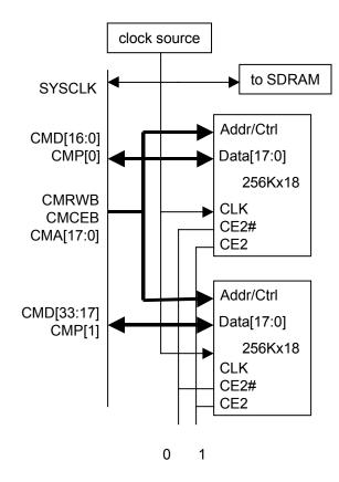
Figure 20 - 1 Bank Configuration for 1MB of Late Write SSRAM
