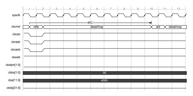
Figure 39 - Power Up and Initialization Sequence
