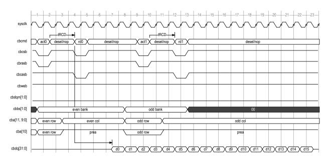
Figure 37 - Write Timing
