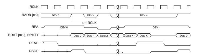
Figure 45 gives an example of the functional timing of the receive interface when configured as a Any-PHY compliant receive master. When S/UNI APEX is capable of accepting at least one more cell, the interface polls addresses until it receives an asserted RPA. As a result, the master re-selects the same RADR again during the last cycle RENB is high to initiate a transfer. If the S/UNI APEX is capable of receiving an additional cell, it will continue to poll for the next available port.
