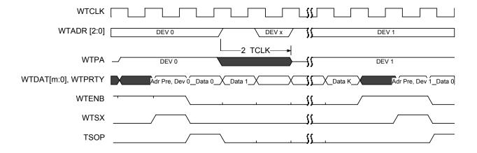
Figure 52 gives an example of the functional timing of the loop transmit interface when configured as a Any-PHY compliant transmit master. The S/UNI APEX
