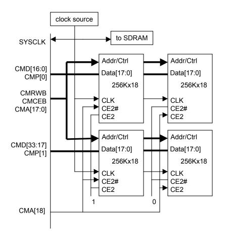
Figure 22 - 2 Bank Configuration for 2MB of Late Write SSRAM
